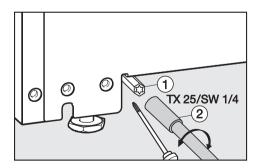
■ If necessary, also align the two rear adjusting devices ① using a socket wrench ②.
